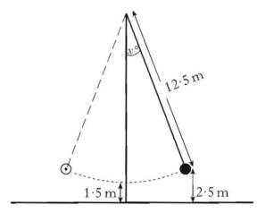
It swings to a maximum height of 2.5 metres above the ground on both sides.
