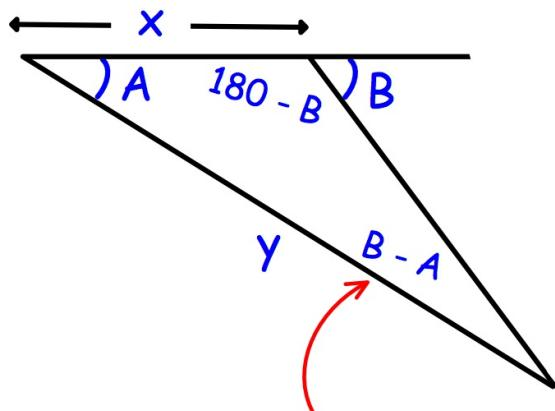
$$\begin{aligned} 180 - (A + 180 - B) \\ = 180 - A - 180 + B \\ = B - A \end{aligned}$$
